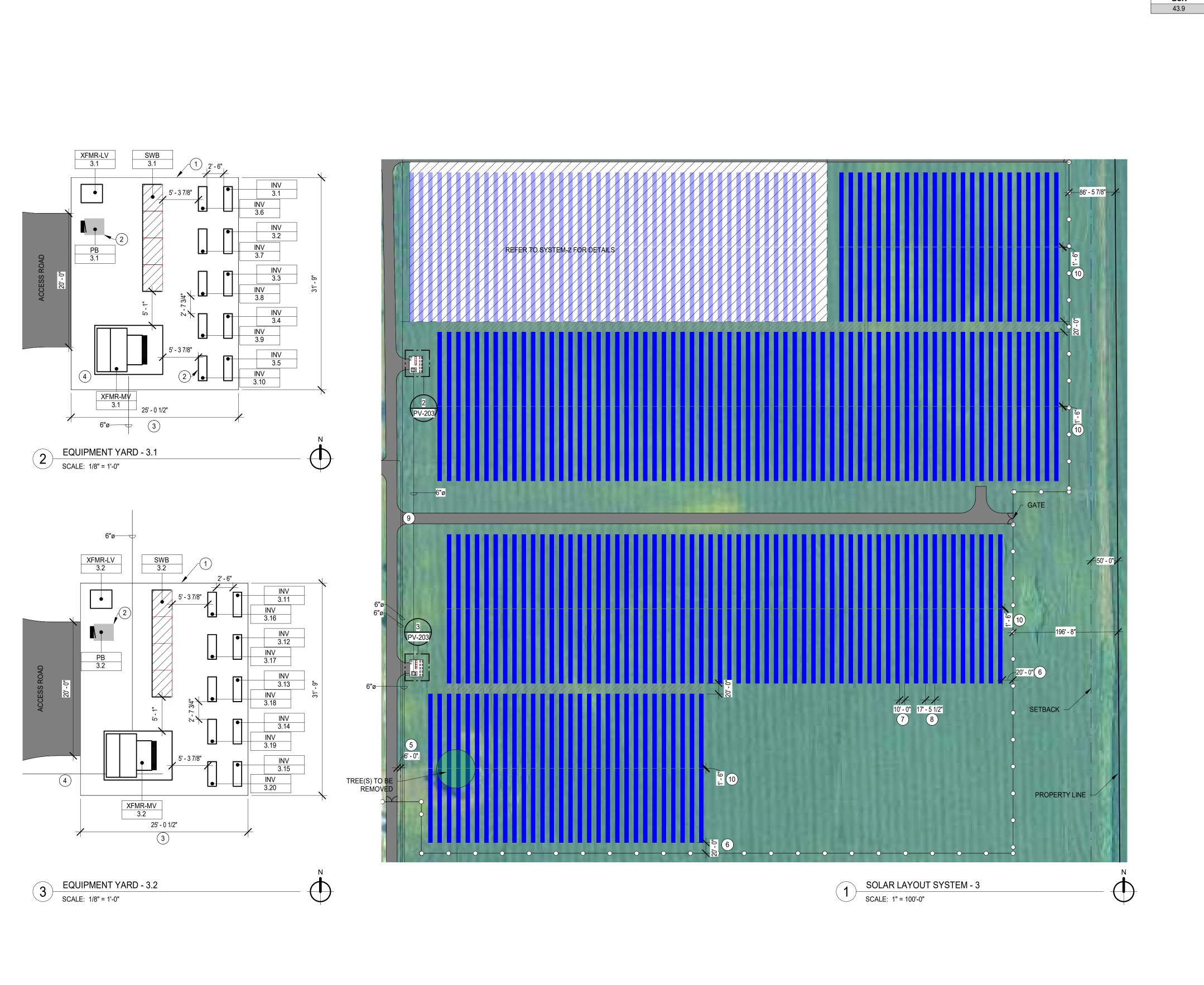
**SYSTEM SIZE - DC SYSTEM SIZE - AC** 7037 kW 5000 kW **INVERTERS** POWER QTY MANUFACTURER MODEL AC VOLTAGE DC VOLTAGE 250 kW 20 SOLECTRIA XGI 1500-250 600 V 1500 V MODULES & STRINGS SIZE MANUFACTURER MODEL QTY STRING SIZE APPROX. # OF STRINGS 540 W WAAREE Bi-55-540 13032 24 543 **TRANSFORMERS SECONDARY** PRIMARY QTY kVA (EACH) SECONDARY VOLTAGE WINDINGS PRIMARY VOLTAGE (POI) WINDINGS 600 V WYE 34500 V DELTA 2 2500 **RACKING** GCR PITCH **RACKING TYPE**
